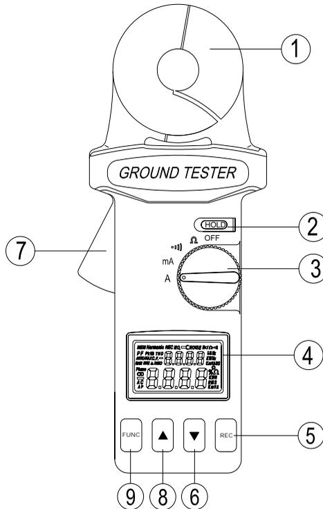
1. Jaws Assembly: Enclose electrode or ground rod. No air gap is allowed between two half jaws.
