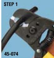
**2** Use an IDEAL coax stripper (45-603 or 45-526) to step-strip coax to proper dimensions.
