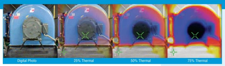
Adjustable Blended View for Ease of Use The HeatSeeker captures both a full infrared image and a digital photo. The thermal image can be overlaid on top of the digital image in various % blends for clarity.
