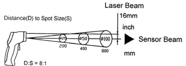
2. Optical Resolution: As the distance from the object increases, the measuring spot size area becomes larger.
